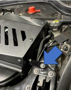
14. You can now reinstall the MAF sensor back into the new pipework using the supplied M4x10mm Socket Head bolts with washers.
