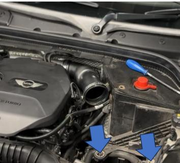
4. Now you can remove the original intake pipe by releasing the retaining clip, as shown below.
