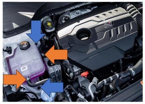
2. Locate the nut attached to the left-hand engine mount and loosen it enough so that the header tank mounting bracket can slide underneath it.
