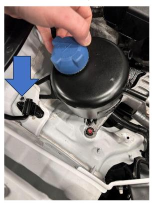
4. Install the supplied M6 bolt and washer as shown onto the bracket to secure. Re-install the hoses onto the header tank and secure with the original clips.
