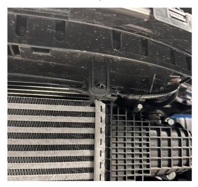
8. Undo the 10mm bolt holding on the upper intercooler bracket each side.
