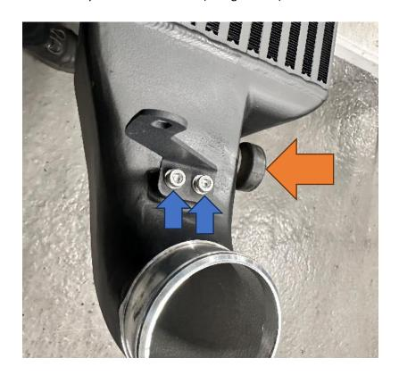
13. Using a second person to help, guide the intercooler into place by seating the rubber mountings into place. onto the car making sure the rubbers seat into their original mounts and install the supplied M6x18mm bolts with washers through the brackets and into the holes where the boost pipes were originally mounted. When happy with the positioning of the intercooler proceed to fully tighten all bolts.
