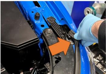
2. Raise the car into the air and remove the two Phillips screws holding the bumper to the arch liner. Then remove the screw on the inside lip of the bumper attached to the wing.
