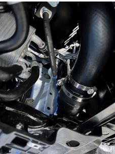
15. Clip the air temperature sensor into the new mounting bracket and then bolt it in place above the intercooler using the supplied M6 bolt, as shown.
