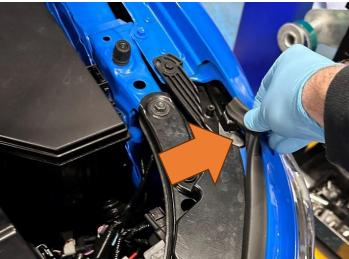
2. Raise the car into the air and remove the two Phillips screws holding the bumper to the arch liner. Then remove the screw on the inside lip of the bumper attached to the wing.
