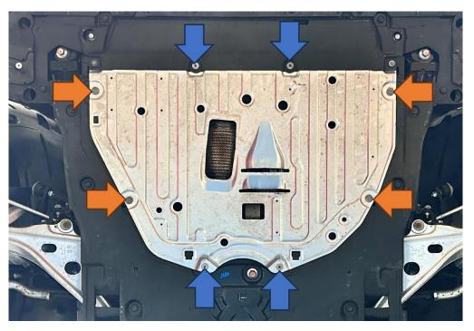
4. At the front, remove the six 10mm bolts (blue arrows), 10 plastic clips (orange arrows) and one crosshead screw (green arrow).
