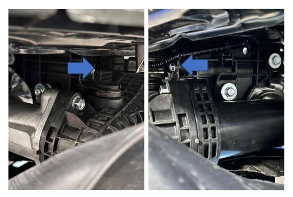
8. Now remove the two 12mm bolts holding the intercooler flange to the boost pipe flange each side and remove the intercooler from the car.
