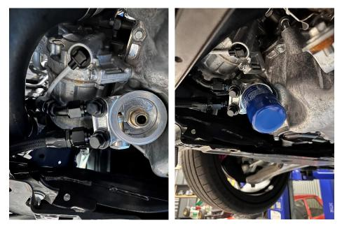
17. Finally, top up the car with 500ml of the manufacturer's recommended grade of oil and then reinstall parts removed in the reverse order that enable you to start the vehicle. Allow the vehicle to run up to temperature and check for any leaks, tightening any fittings as necessary. Once cool, check the oil level and top up as required. When happy with the install you can then reinstall the remaining parts in reverse order of removal.
