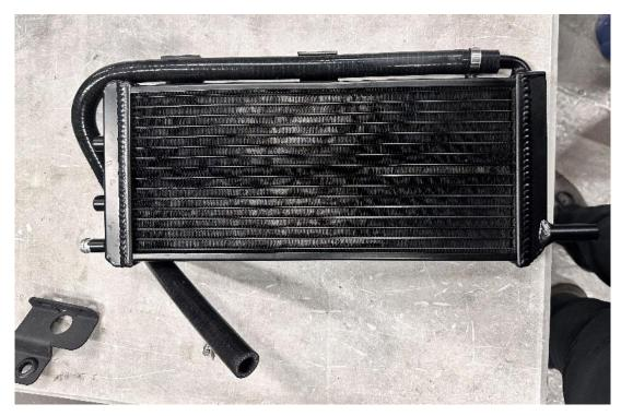
6. Now position the radiator in the car. The lower locating pin slots into a hole in the bottom of the radiator pack. Once in place, you can then install the new mounting bracket by locating the pins into the rubber bushes before reinstalling it with the original bolts. **Please note:** Take care not to damage the original radiator whilst you position the turbo radiator.
