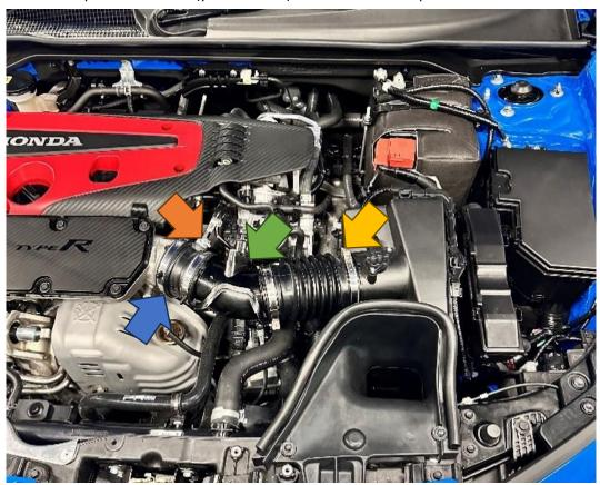
8. Now locate the original coolant hose (blue arrow) and using hose clamp pliers, remove the clip and hose from the take-off. The new hose (orange arrow) can now be fitted in its place with a jubilee clip.
