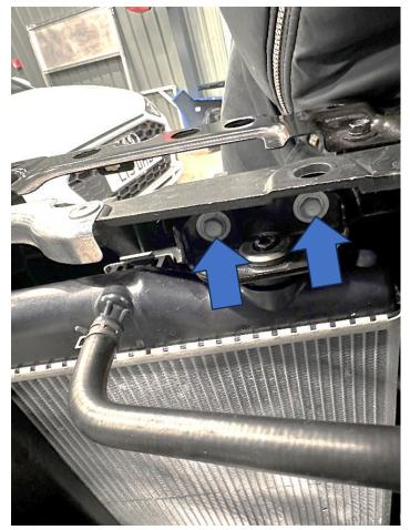
4. Remove the rubber bush from the original radiator bracket (blue arrow) and install it onto the supplied mounting bracket along with the two supplied rubber bushes (orange arrows).
