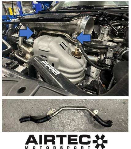
13. Install the second silicone hose onto the car as shown using the supplied jubilee clips. Once happy with the positioning of both hoses, proceed to fully tighten the jubilee clips.
