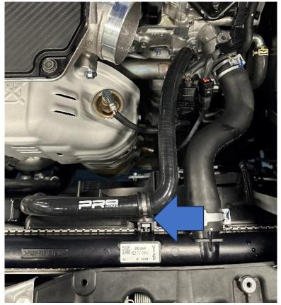
10. To fit the second silicone hose, you will need to remove the two 10mm bolts holding the wiring harness and vacuum hoses to the inlet pipe. Then move it back and disconnect the plug to the turbo actuator.
