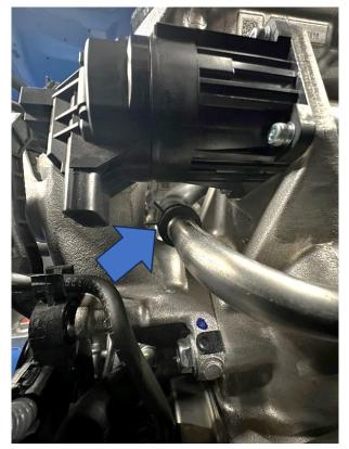
12. To remove the section of hose from the vehicle, you will need to remove the two 10mm bolts holding the pipe work to the inlet manifold. This can then be removed from the car, which will take the hoses at both ends with it.
