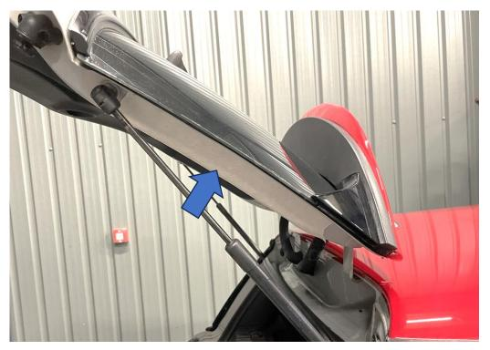
2. With the help of someone, hold the correct sided bracket up against the boot lid as shown.
