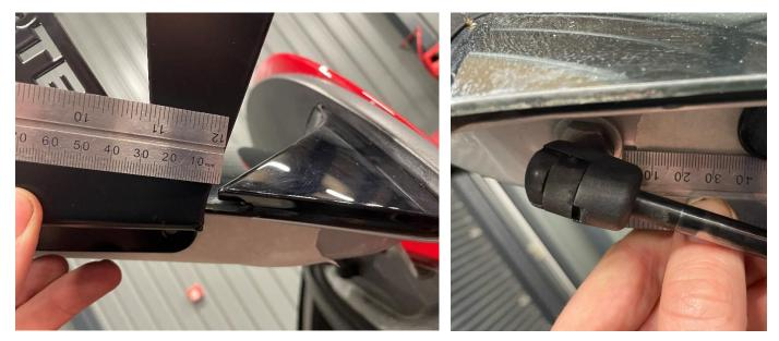
4. Now mark the three mounting holes and remove the bracket.
