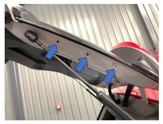
6. Now attach the bracket by bolting it in place using the supplied bolts with washers.
