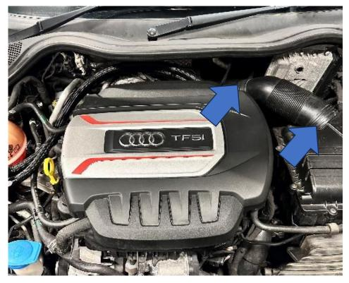
2. At the back of engine, locate the turbo's outlet hose and using a jubilee flexi-driver or flat-bladed screwdriver, undo and remove the standard hose attached to it.
