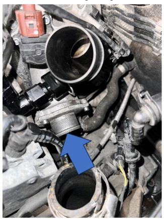
4. Finally, install the supplied rubber gasket onto the AIRTEC Motorsport turbo muffler delete and insert it into the turbo. Reuse the original bolts and then reinstall the hose and induction pipe in reverse of removal.
