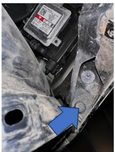
4. With the help of a second person, carefully but firmly pull the bumper out from each corner and then remove it from the car.
