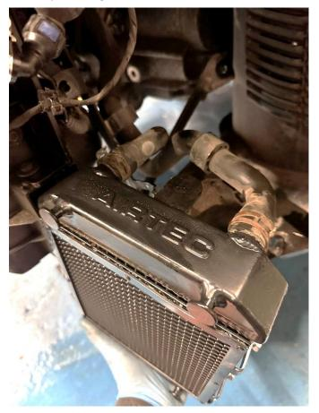
12. Install the radiator into the rubber bushing before lifting the bracket hook back into place and reinstalling the three bolts removed in Step 7.
