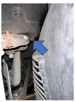
8. Lift the radiator up so the top bracket unhooks.
