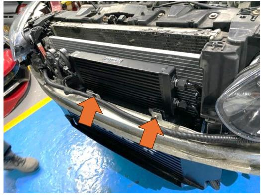
8. Tighten the connections to the oil cooler and then route the lines behind the crash bar and under the radiator pack towards the oil filter.
