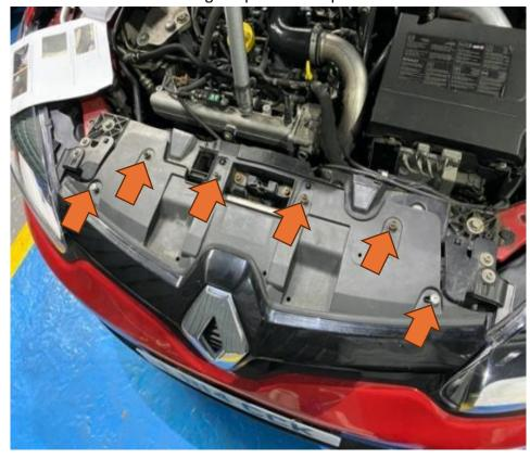
2. Remove the two T20 Torx bolts from inside the inner wheel arch liner and then remove the five plastic clips to enable more room to remove bumper.
