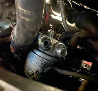
10. You can now connect the oil lines to the sandwich plate. Make sure they are fully tightened before refitting the oil filter.
