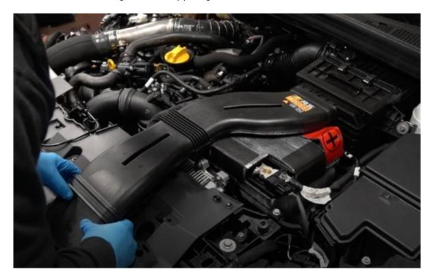
2. Release both the positive and negative battery terminals using a 10mm socket then release the 10mm bolt securing the fuse box in place to the left of the battery.
