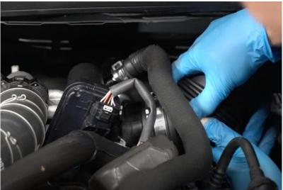
8. Remove the two hoses from the turbo intake pipe using a hose clip pliers or similar. You will then have access to the two 13mm bolts which will need to be removed in order to remove the turbo pipe
