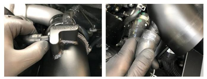
11. Place the supplied spacer where the original air box bolt was located, as shown. Then fit the base of the induction shield in place using the supplied M6x90mm bolt with a washer down through the spacer.
