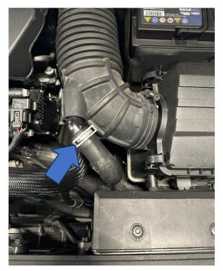
2. Unclip the hose clamps holding the two hoses at the rear of the intake pipe and then remove the hoses by giving them a firm pull.
