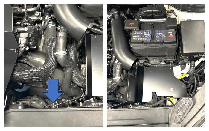
13. Install the rear part of the shield using the four plastic push fits provided.
