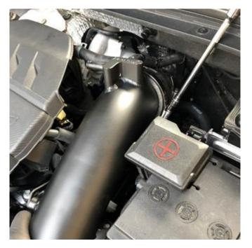
9. Using the supplied M6x12mm Socket Head bolt and a large washer, attach the bracket fitted in Step 7 to the mounting boss on the side of the intake pipe. Leave the bracket slightly loose so the pipe can be positioned correctly once the air filter is on.
