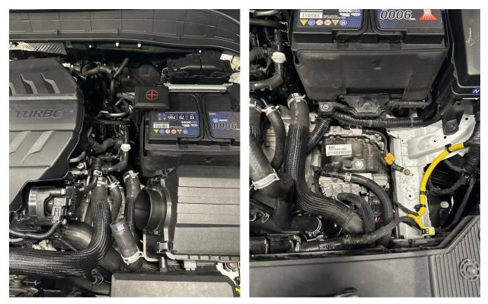
7. Locate the 10mm bolt on the side of the cylinder head highlighted and loosen it until you can slide the longer of the two supplied mounting brackets behind it. Position the bracket roughly as shown and then tighten the bolt to hold the bracket in place, but not fully to allow adjustment later.
