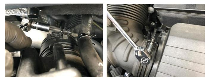
4. To release the front section of the air box, remove the two 10mm self-tapper bolts that screw into the slam panel, as shown.
