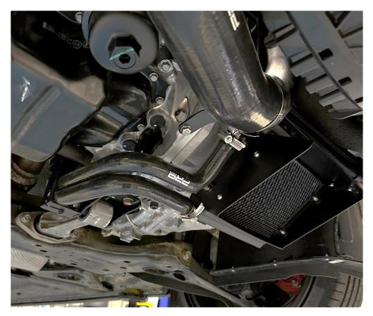
14. Finally, reinstall the lower plastic tray in reverse of removal and then top up the coolant and follow the manufacturer's recommendations for bleeding air out of the system. Check the system for leaks once the car has cooled down and tighten any fittings as necessary.
