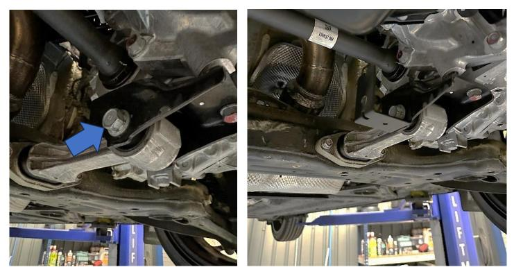
6. Locate the spare bolt hole boss in the front of the gearbox, as shown and install the upper radiator bracket in position using the supplied M8x16mm Socket Head bolt with a washer, but do not fully tighten at this stage to allow for adjustment.
