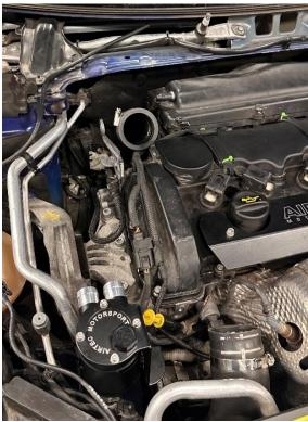
6. Working on the other side of the engine bay, move the air feed by lifting it up and over so you can gain access to loosen the jubilee clip underneath for the boost hose from the bottom of the turbo. Then follow the hose down and disconnect the plug clipped to the dump valve.
