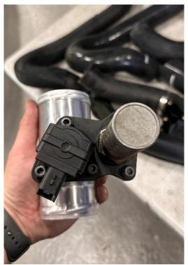
10. Install the smallest silicone hose onto the turbo and tighten the jubilee clip so that it keeps it in place but t can still rotate if needed. Then install the alloy joiner with the dump valve with a jubilee clip. You can then install the next silicone hose going to the intercooler (shorter U-bend) with jubilee clips and once happy with the fitment, fully tighten all clips and reconnect the dump valve plug, as shown.
