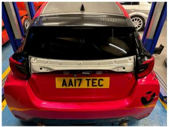
5. Hold each of the uprights up to the boot lid and mark the three holes. **IMPORTANT:** Make sure the uprights measure approx. 6.5mm away from the glass and are **exactly** the same both sides before marking.
