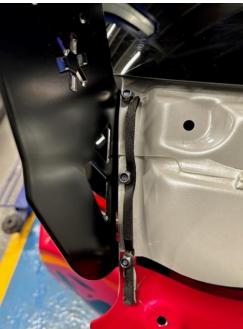
8. Once fully tightened, refit the exterior trim in reverse of Steps 1 to 4 and carefully close the boot lid, as the uprights are not fully aligned yet.
