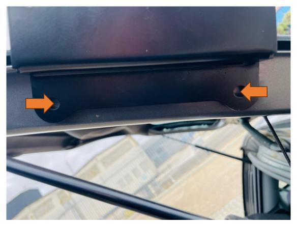
4. Starting with a 4mm drill bit, make the holes using the guide marks you made and then use a 9mm drill bit to increase the hole size so that the rivet nuts will fit.
