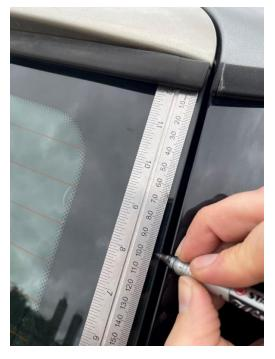
2. Open the boot and using the correct side bracket (two holes at the bottom, one at the top) line up the top of the bracket with where the mark made in Step 1, as shown. Using masking tape, temporarily fix the bracket in place and then double check the height with the ruler to confirm the bracket starts at 100mm.
