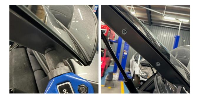
6. Now fit the supplied spacer in place each side before attaching the brackets onto the car using the supplied M6 Hex Head bolts with Mudguard washers.
