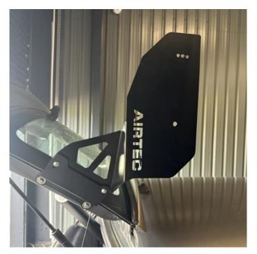
8. Using a second person to help, attach the supplied wing blade to the vehicle in your desired fixing location.
