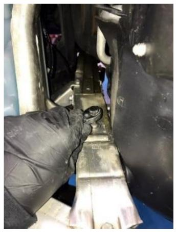
10. You can now remove the front lower crossmember from the car and place it out of the way.
