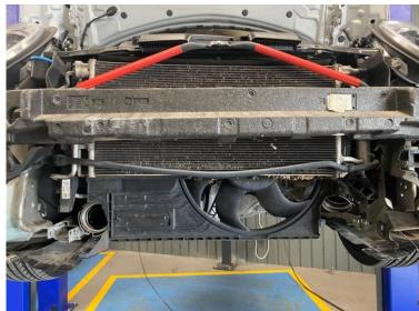
14. Using a small screwdriver, hold up both sides of the rad pack, as shown.
