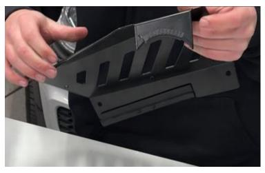
8. Install the side bracket using the supplied M6x16mm Button Head bolt with a Nyloc nut and washers both sides, but do not fully tighten yet to allow adjustment later on. Then attach the two CNC push fits onto the base of the air box, using two more M6x16mm Button Head bolts with washers and spacers
