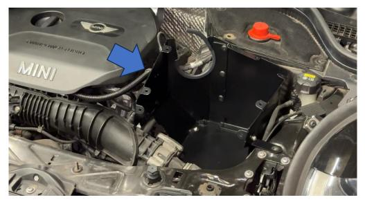
12. Now install the MAF pipe work with the air filter into the silicone hose and secure in place using the supplied 80mm jubilee clip.
