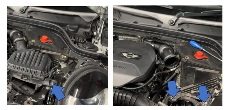
4. Now you can remove the original intake pipe by loosening the jubilee clip, as shown below.
