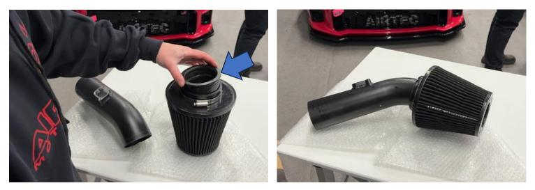
10. Install the supplied 80mm silicone hose with jubilee clip onto the original crossover pipe, but do not tighten to allow adjustment later on.
