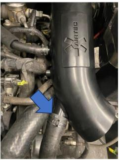
8. Remove the 10mm bolt shown in the picture below, then install the supplied bracket and refit the bolt. Then attach the bracket to the alloy pipework using the supplied M6x12mm Hex Head bolt with washer.
