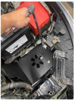
10. You can now install the air feed, which will secure to the side of the heat shield using the two push clips supplied. Then you can fully secure the air feed in place by installing the two fir tree clips through the top of the air feed into where the original one was located.
