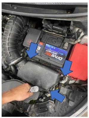
4. The air box can now be removed from the engine bay. Whilst removing, unhook the original air feed from the slam panel.
