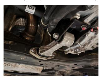
3. Undo the 17mm boltt holding the torque mount to the bracket.
