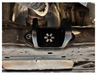
6. Install the torque mount body onto the base using the supplied M12 bolt, noting the orientation from the picture below.
