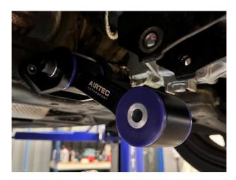
7. Finally, re-install the original 17mm bolt removed in Step 3, making sure to install the supplied spacer between the bush and the bracket.
