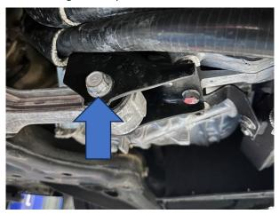
4. Undo the two 14mm bolts holding the torque mount base to the body of the car.
