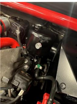
4. Install the longer hose onto the take-off next to the oil cap, as shown and then onto the take-off pointing towards the front of the car with two of the jubilee clips supplied.
