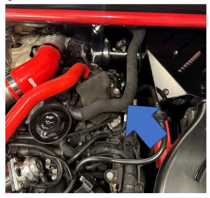
2. Remove the hose from the car by loosening the securing clips at both ends. If you have the AIRTEC Motorsport induction kit fitted, you will also need to remove the short 90-degree silicone hose attached from the original hose to the induction hose.
