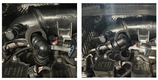
4. You can run the kit without an engine cover if you prefer however, if you would like to reuse your engine cover then a hole will need to be made so that the hose can connect back onto the engine. Make a mark at the measurements shown below and then use a drill to make a pilot hole before using a 32mm hole saw. The engine cover can then be reinstalled.
