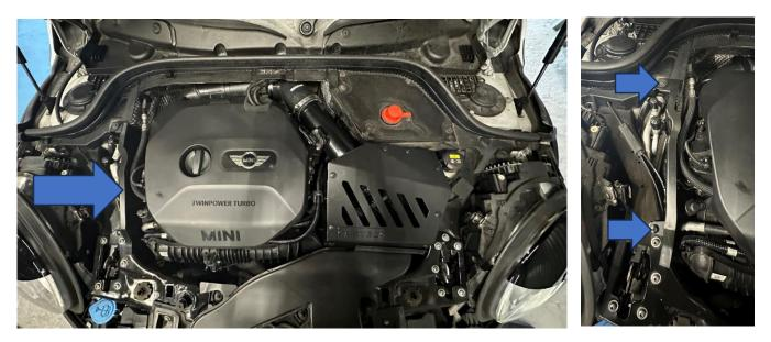
2. Pull the engine cover up from the lower left corner to remove.
