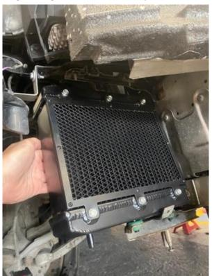
12. Once the new radiator is in place, you can reinstall the two coolant hoses in revers of removal.
