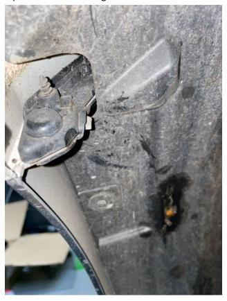
5. Carefully pull back the weather strip along the top of the bumper and remove the six T30 bolts underneath.
