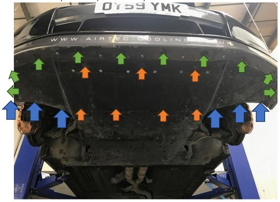
4. Remove the front section of the inner arch liners by removing the one Phillips screw and six push fittings each side.
