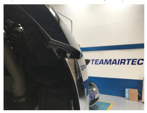
6. Now remove the three 10mm bolts securing the bumper to the wing.
