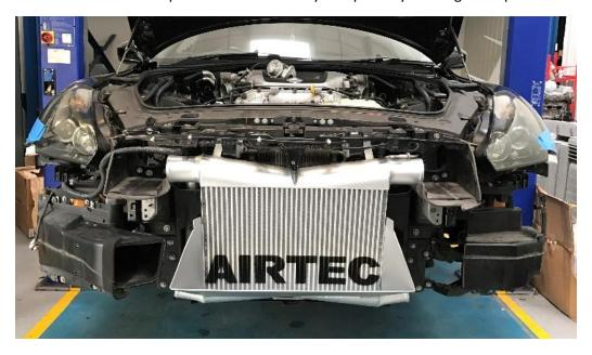
Fit the boost passenger side boost hoses, as shown. Please note: the washer bottle support bracket may require trimming for clearance on the silicone hose.
