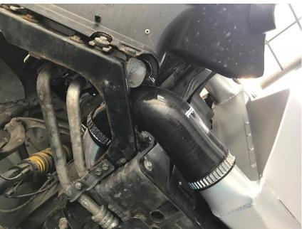
18. Now fit the replacement induction pipes. The driver's side is secured with the original 10mm bolt as shown. Then attach the passenger's side with the original 12mm bolt as shown and attach the filter.
