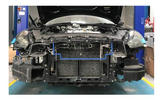
13. The original intercooler lower mounting bracket needs to be removed using a Dremel tool or similar. Then locate the supplied lower intercooler mounting bracket by bolting it from underneath using the supplied bolt and washer (orange arrow). With the bracket in place, mark the two facing holes (blue arrows). Then remove the bracket, drill the holes using a 9mm drill bit, insert the supplied Riv Nuts and refit the lower bracket.
