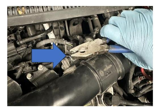
6. Place the new AIRTEC Motorsport pipe into position but before securing, refit the take-off removed in Step 3 onto the pipe in the same position. Make sure you press the green button and carefully but firmly push it on until it clicks. Then refit securing clip into place.
