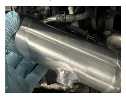
8. Locate the pipe into position and secure the left-hand side onto securing post first.
