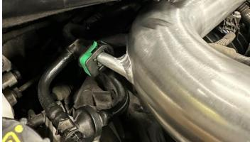
7. Now refit the vacuum line removed in Step 5 in reverse of removal.
