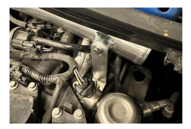
10. Finally, refit the primary and secondary intake hoses in reverse of Steps 1 to 2 and then check all clips, fittings and bolts are secure.
