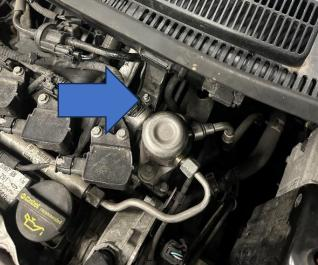
5. Once unbolted, the top pipe can be removed from the securing posts and gently pulled forward to give access to the vacuum line at the back on the right-hand side. Use some pliers to the release the retaining clip and disconnect the line from the pipe. The pipe can then be removed from the engine bay.
