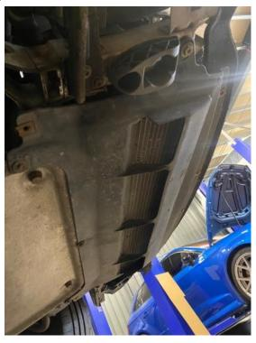
2. Now you will be able to access the three 13mm bolts which will need to be removed to allow the oil cooler to drop down. **Only loosen these** as it will make it much harder to remove the oil lines if they are fully removed.
