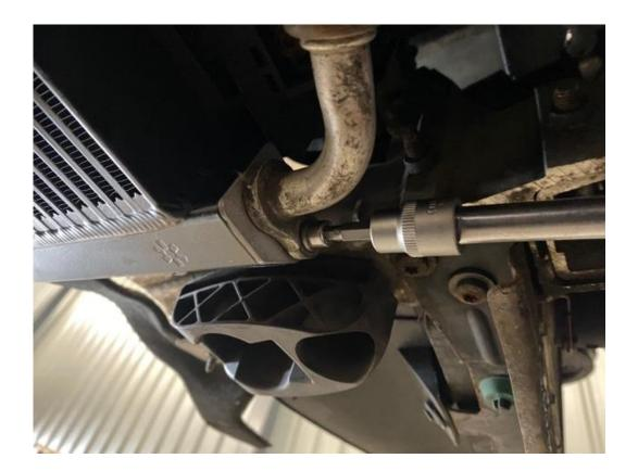
8. Now you can fully tighten the three 13mm bolts to fully secure the oil cooler in place.
