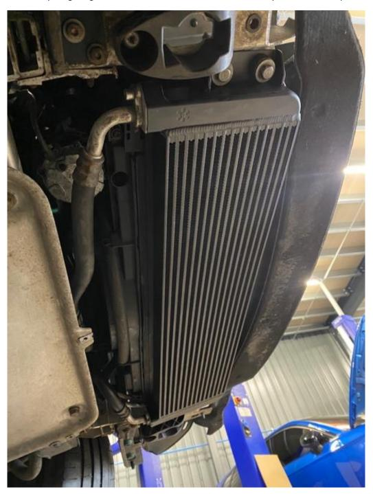
10. **IMPORTANT:** Finally, top up the oil. You will need approx. 500ml but check the level before filling and start the car. Look immediately for leaks from any of the connections. If there are, turn the engine off, retighten the fittings and repeat. Then let the car get to full operating temperature, recheck the oil level and top up if required.
