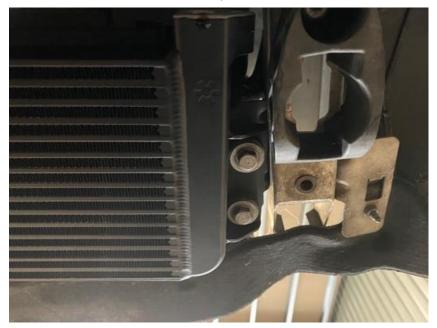
6. At this stage, check the alignment of the pipe fitting onto the new oil cooler. In some cases, the holes on the pipe fitting may need elongating to allow the bolt to locate.
