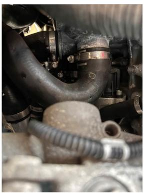
14. Install the breather pipe removed in Step 8 onto the CNC fitting take off using the supplied M4 hardware to secure. Then install into the silicone hose using the smallest jubilee clip supplied and fully tighten.
