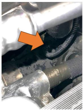
8. Now unclip the top of the breather hose from the engine by lifting the tabs carefully whilst applying pressure to pull the hose away from the engine. Once unclipped, remove the hose from the car.
