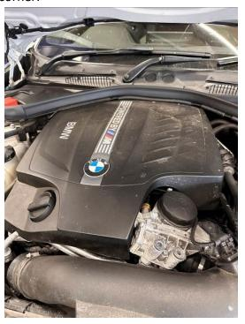
2. Undo the hose clamp to the induction pipe on the left-hand side.
