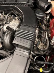
2. Remove the four bolts on each throttle body using a 5mm Allen Key and undo the lowest/bottom jubilee clip. This will allow the elbow and hose assembly to be removed as one. The elbows are tightly held in place due to the O-rings, so first pull the elbow away from the plastic flange and then up and out of the engine bay.
