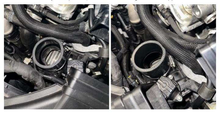
6. Next, place a jubilee clip over the silicone hoses and install the AIRTEC Motorsport elbows down into them. Once at the correct height, locate the flange onto the throttle body, making sure the O-ring is seated correctly. Then use the provided 5mm Allen Key and bolts to secure the pipes in place.
