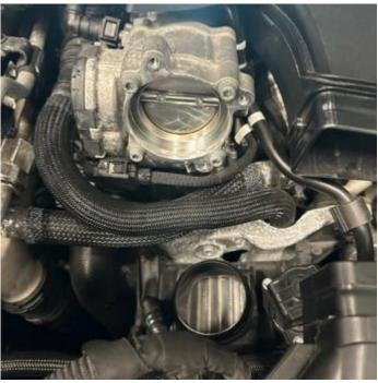
4. Next, remove the O-rings from the plastic flanges, as these are reused in the AIRTEC Motorsport elbows, as shown. Be careful when removing the O-ring from its groove, as it's important not to cut or scratch them otherwise they will not seal properly.
