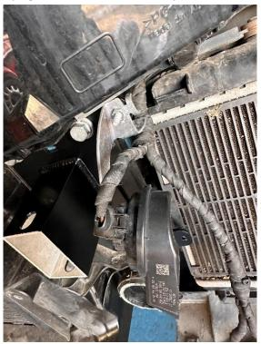
18. Install the lower bar onto the intercooler using the supplied M6 bolts with washers, as shown. These brackets are slotted so that if needed you can adjust the position of the bar once it is on the car.
