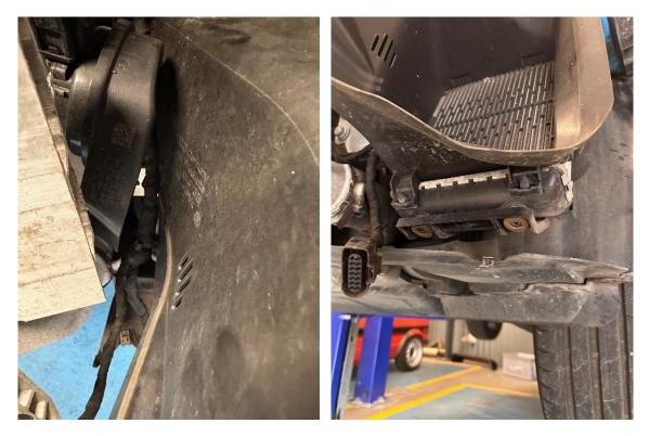
10. Unplug the horns by squeezing the connectors and then unclip the wiring loom connected to the crash bar.
