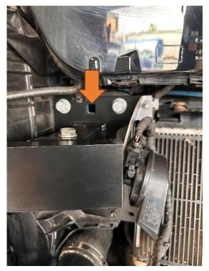
22. Install the temperature sensor into the bracket attached to the intercooler.
