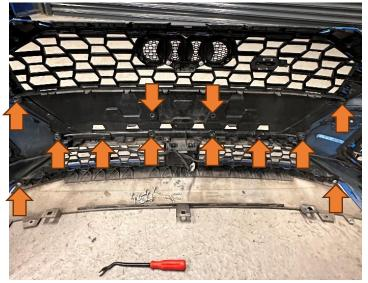
27. With the grille removed, we recommend cutting along the ridge of the plastic, as shown. Use a suitable cutting tool, however it is up to you how much you want to remove exactly.
