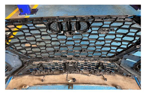
29. Finally, refit the auxiliary radiator surround and bumper in reverse of Steps 1 to 14, making sure to reroute the far side washer jet hose back into place.
