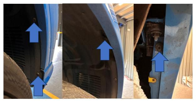
5. Feeling inside the wheel arch, underneath the liner you will be able to feel the clip for the bottom of the outer wheel arch trim. Squeeze this together as you gently pull on the bottom of the trim to release it and then work your way round until you have enough removed that the corners of the bumper would be free to come out.
