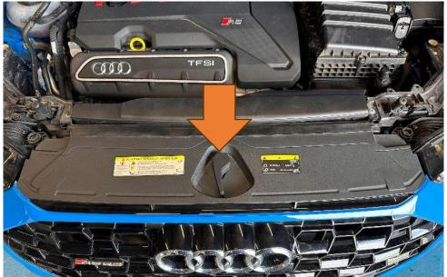
3. Now pull the plastic slam panel from the edge and then remove from the vehicle, this will reveal two T25 screws that you will need to undo.
