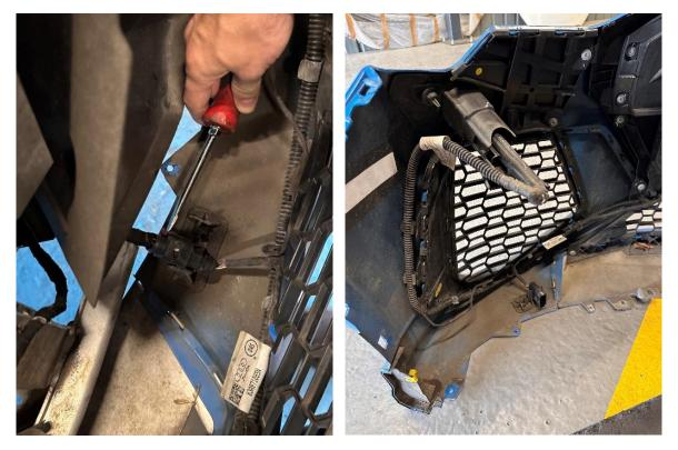
8. Remove the temperature sensor from the crash bar by squeezing the front as you pull the back of the sensor and then unclip the loom from the lower crash bar leg.
