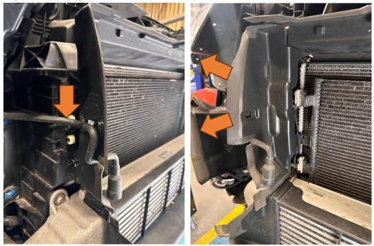
14. Undo the two jubilee clips to release the silicone hose connectors followed by the two T27 bolts holding the top of the intercooler in place. You can now tilt the intercooler forwards and lift it to remove it from the car.
