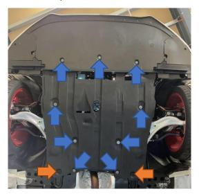
3. Using a trim tool, remove the four plastic clips highlighted in each arch liner and remove the section from the car.
