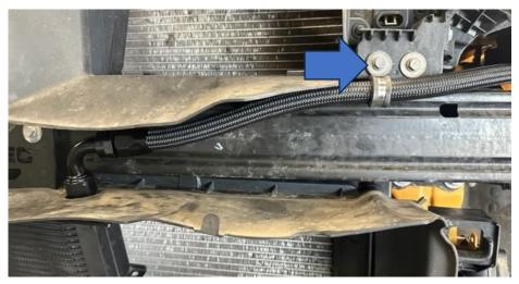
13. Working under the car, locate the original oil cooler modine above the oil filter. You will need to remove the two coolant lines attached to it using hose clamp pliers (or similar) and then insert the supplied alloy pipe joiner between them to link the hoses, reusing the original hose clamps, as shown. We recommend clamping the lines to lose minimal coolant.
