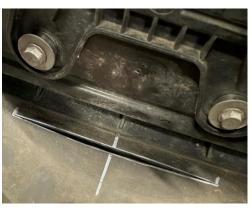
10. Undo the two 10mm bolts and washers located above the cut and insert the supplied AIRTEC Motorsport bracket through the gap created. Then reinstall the bolts with the provided spacers mounted behind the new bracket so it sits level, as shown.
