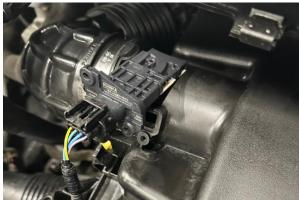
3. Now, use a trim removal tool to unclip the MAF cable and move it aside.
