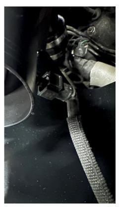
19. Install the induction pipe bracket using the supplied M6x16mm Button Head bolt and Nyloc nut with to install to the shield first and then attach the bracket to the pipe using the other M6x16mm Button Head bolt. When happy with the position of the pipe fully tighten the bolts.
