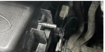
2. Unbolt the MAF sensor housing using a T20 Torx and then unplug the MAF sensor by squeezing the tabs and pulling it apart.
