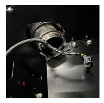
15. Install the 35mm P-clips around the bar at the back of the engine bay and attach to the induction shield using the supplied M6x16mm Hex Head bolts with washers and Nyloc nuts, as shown. Use the supplied M6x16mm Button Head bolts with Pan Washers to secure the front lip of the induction shield to the plastic fittings inside the rubber bushes, as shown.
