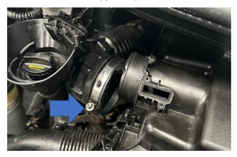
5. Pull up on the front corners of the original air box to release it from the rubbers at the front of the engine. If the rubbers come out with the air box then put them back into their holders as they are reused later.
