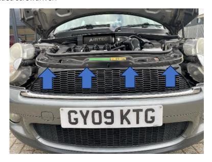
2. Now locate the two outer clips on the bottom of the grille as shown. Gently push these inward whilst pulling on the outer corner of the grille to release. Take care as they can become brittle over time and snap.
