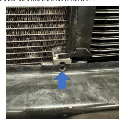
27. Install both the lower brackets facing towards the front using two of the supplied M6x16mm bolts with Nyloc nuts and washers both sides, as shown. Then install onto the crash bar using the last two M6x16mm bolts with Nyloc nuts and washers.
