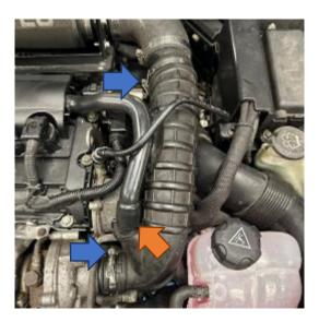
16. Undo the two clamps holding the boost pipe to the turbo and remove from the car. 17.
