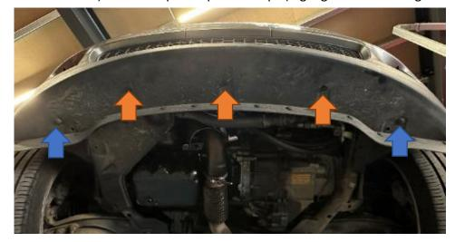
6. Each side, remove the three plastic push fit clips in the wheel arch and pull the liner back to reveal a push fit clip that holds the outer arch trim in place. Remove these to then gain access to the T25 Torx bolt holding the bumper underneath the headlight.
