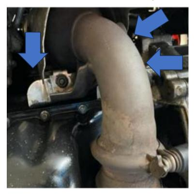
10. Working in the engine bay, now remove the top lambda sensor from the manifold.
