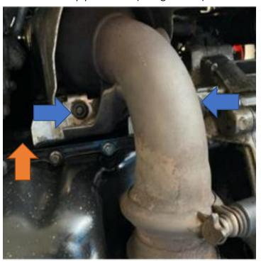
14. Working back in the engine bay, remove the 8mm bolt holding the header tank in place and lift it to release it from the push fit below in order to gain better access. The move it aside and secure as necessary.
