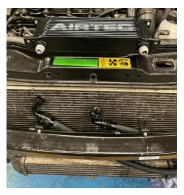
25. Locate the oil cooler in place using two of the original push fits from the upper grille (removed in Step 1) to hold it in place temporarily.
