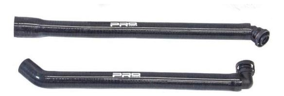
8. Remove the original breather hose by pulling firmly but carefully at each end to release it.
