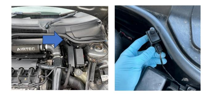
2. Remove the sensor from the bracket by squeezing the back of it and then angling it to release it. The image below shows it with the bracket removed to highlight the part that needs to be pressed.
