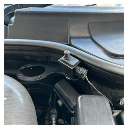
6. Install the catch can using the supplied M5x12mm Socket Head bolts with washers.
