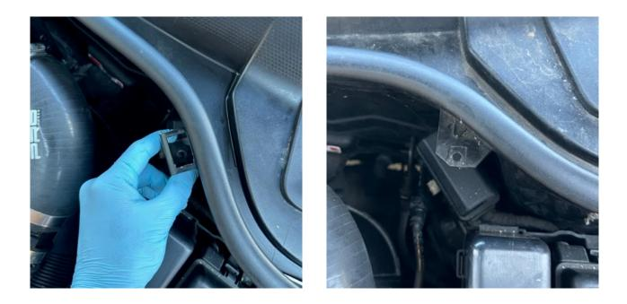
4. Install the AIRTEC Motorsport catch can bracket underneath the original bracket and then reinstall the bonnet sensor bracket on top, as shown. Then secure in place using the supplied M5x20mm Socket Head bolt with a Nyloc nut and Mudguard washers both sides.
