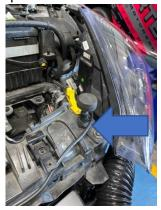
5. Install the MAF boss into the induction pipe using the provided jubilee clip and install your MAF senor in place using a 3mm Hex Key. You will also need to slide the small silicone piece onto the end of the boss in preparation of installing the air filter.
