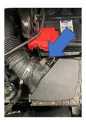
2. Undo the jubilee clip attaching the air box to the induction hose and pull it free. Then firmly but carefully pull the air box to the right to release it from the front air feed and then up to release it from its rubber mounts. Lift the air box out of the engine bay and place aside.
