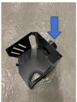
4. Place the new air box into the engine bay by inserting the induction hose (uprated AIRTEC Motorsport induction hose pictured here) through the rubber seal, making sure you push the wiring through at the same time. Also move the bonnet latch cable to the other side of the bonnet stop as shown below.
