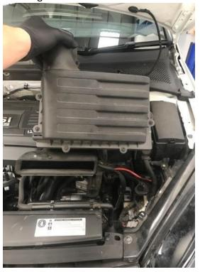
4. You can now install the new intake pipe and secure in place using the supplied jubilee clip (pictured here with our optional uprated Pro Hoses silicone connector).
