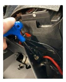
6. Remove the T25 Torx Bolt from the back of the radiator pack and then attach the supplied mounting bracket and re-install the bolt. You can then attach the bracket to the air box base with the supplied M4 nuts, bolts and washers either side.
