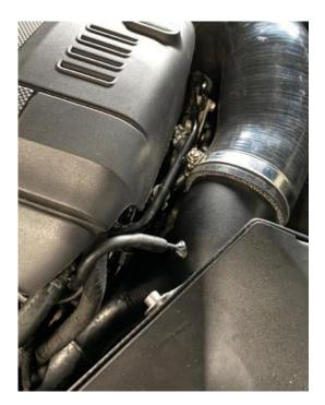
8. Finally, install the enclosed air box lid by placing it on top of the base and align the tabs with the allocated holes. You can now secure the lid using the supplied push fittings. Then check everything is aligned, tight and secure.
