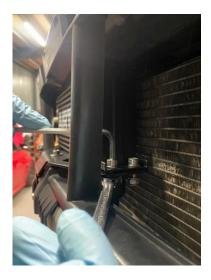
10. You can now feed the oil lines up to the sandwich plate. Secure the first oil line to the top fitting before securing the lower fitting in place, as shown. Once they are secured correctly you can cable tie the oil lines together to make sure they do not rub on any other pipework.
