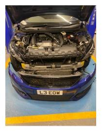
4. You will need to remove the intercooler. Loosen the jubilee clips from both ends of the and then remove the hoses. Once the hoses have been removed you can release the two 13mm bolts from the brackets securing the intercooler in place.
