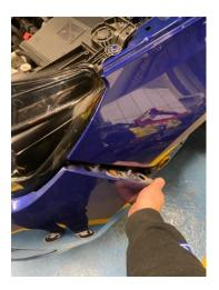
3. You can now remove the seven remaining 10mm bolts from underneath the front bumper. After they have been removed, unplug the two wiring harnesses and remove the bumper.
