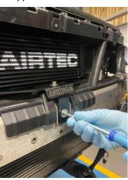
9. The oil cooler can now be secured to the bracket with a 5mm Allen Key and 10mm spanner.
