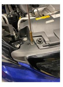
2. Remove the two T30 Torx bolts and an additional plastic clip in the arch liner then pull it away and remove the 10mm bolt holding the wing to the bumper.
