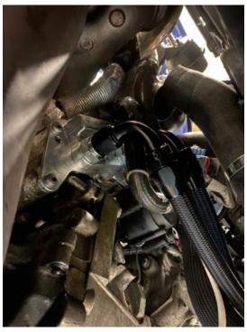
18. **IMPORTANT:** Finally, top up the oil (approx. 500ml) and start the car. Look immediately for leaks from any of the four connections and the oil filter. If so, turn the engine off and retighten the fittings if needed. Then let the car get to full operating temperature, recheck the oil level and top up if required. Once the level is correct, refit the bumper in reverse of removal.
