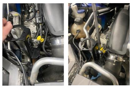
2. You can now attach the oil catch can to the bracket using the supplied bolts and washers and secure using a 4mm Allen Key.
