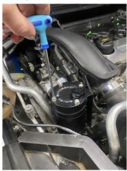
3. Remove the original breather pipe from the vehicle by applying pressure onto both sides of the fitting and then pulling to remove. On the other end of the breather pipe, you will only need to pull it from the hose to remove.
