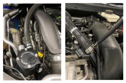
5. The second hose can then be installed onto the left-hand side of the catch can. Follow the hose up and round in line with the first hose. This will secure using the push fitting onto the engine where the original hose was fitted.
