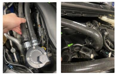
6. Finally, you can now secure the hoses together using the supplied cable ties and check that everything has been secured correctly.
