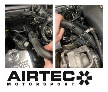
4. Now install the longest piece of pipework by installing the push fitting onto the right-hand side of the catch can. The hose can then follow up and over the engine bay and down onto the original induction hose. The silicone can then be secured using the provided jubilee clip.
