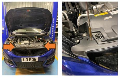
2. Remove the two T30 Torx bolts and an additional plastic clip in the arch liner, then pull it away and remove the 10mm bolt holding the wing to the bumper.
