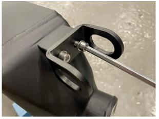
6. Fit the new intercooler in place by reusing the original fittings and reattach both hoses.
