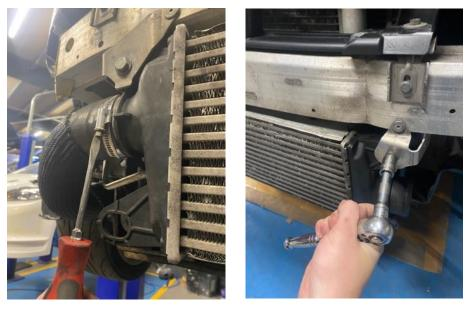
5. Now attach the AIRTEC Motorsport mounting brackets to the top tabs of the new intercooler using the bolts and washers supplied, as shown.
