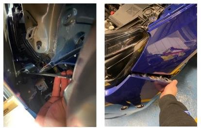
3. You can now remove the seven remaining 10mm bolts from underneath the front bumper. After they have been removed, unplug the two wiring harnesses and remove the bumper.
