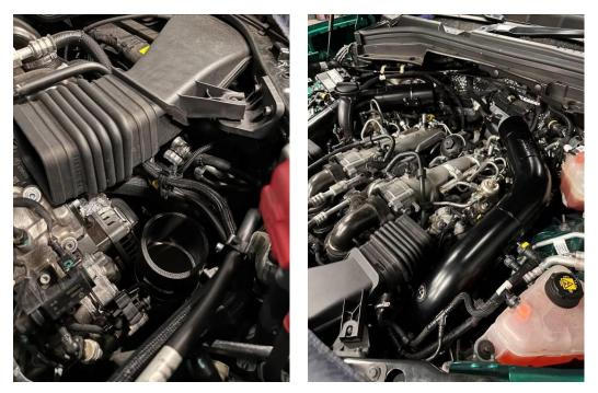
10. Now fit the lower air guide and mounting brackets using the supplied M6x16mm Socket Head bolts with washers, as shown. Then install the new induction pipes using the supplied M6x12mm Socket Head bolts to attach to the brackets to the pipes, but do not fully tighten the bolts at this stage.
