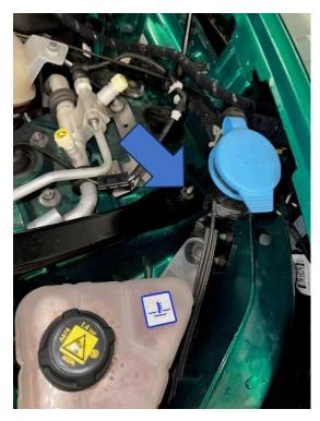
2. Open the bonnet and remove the engine cover by carefully but firmly pulling up from the back corners to release it from its mounts.
