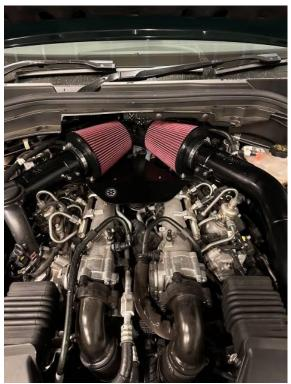
12. Clip the vac line connectors back onto the pipe, you will hear a positive 'click' once fully inserted.
