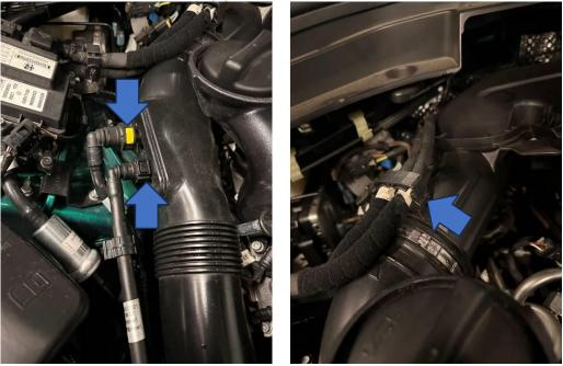
4. Disconnect both the clips attached to the front of the original pipework.
