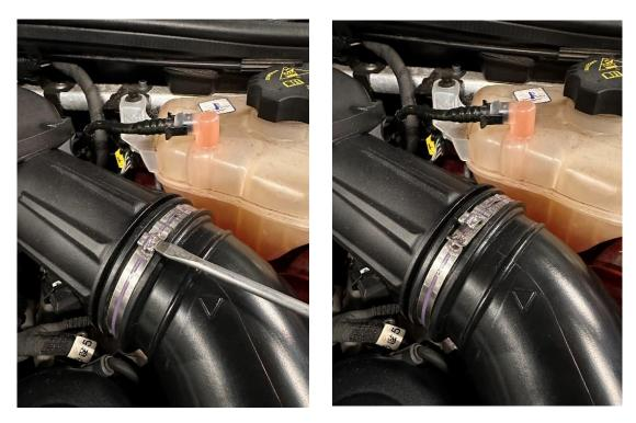
6. Push back the rubber joiners from the air feeds at the front and then remove the original air box from the car by firmly but carefully lifting the corner and pulling it from the rubber mounts. As you remove it, you will need to disconnect a wiring clip on the left-hand side an unclip a small pipe from the right-hand side.
