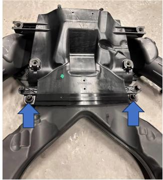
14. Finally, install the supplied upper air guide using the M6x60mm Socket Head bolts with washers and place the supplied spacers between the upper and lower air guide, as shown. The reinstall the strut brace in reverse of removal.
