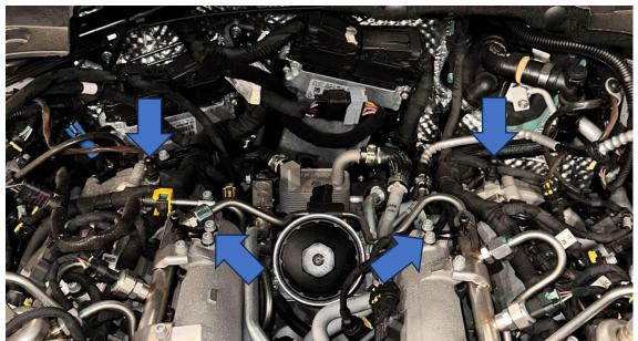
8. Fit the supplied brackets reusing the original bolts and then install the supplied threaded spacer onto the front mounting studs, as shown.
