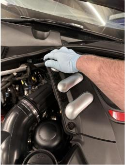
2. Locate and unclip the vacuum lines each side (four in total) attached to the original pipes by squeezing the tabs each side and pulling.
