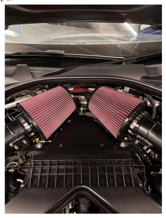
13. Finally, install the supplied upper shield using the supplied M6x12mm Socket Head bolts with the last two spacers and tighten.
