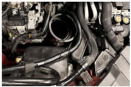
10. Now insert your new AIRTEC Motorsport induction pipes into the silicone connecters but don't tighten the second set of jubilee clips yet. Attach the top brackets to the pipework using the supplied M6 bolts and washers (two each side) but do not fully tighten yet. Then reconnect the original vac lines removed in Step 2 by pushing them on until you hear a positive 'click'.
