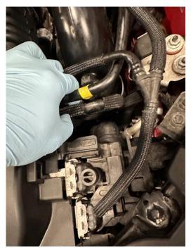
4. Release the two retaining clips from the pipes connected to the air box using a flat-bladed screwdriver to get into the gap in the clip and twist. There are two more clips at the bottom of the pipes to undo; you may need a torch to see them. The pipes can then be removed.
