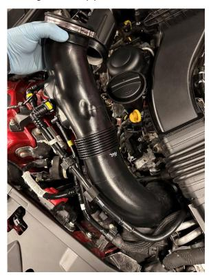
6. Push back the rubber joiners from the air feeds at the front and then remove the air box from the car by firmly but carefully lifting the corner and pulling it from the rubber mounts.
