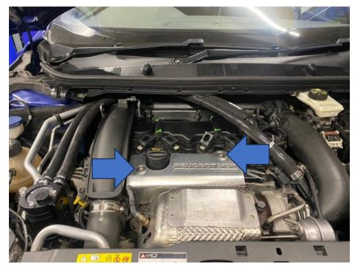
2. Now fit the new plate in place using the supplied bolts, washers and spacers. Use two spacers on the left-hand side and one on the right-hand side.
