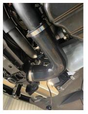
17. Secure the air-con radiator onto the AIRTEC Motorsport intercooler by using the provided brackets that mount directly onto the threaded bosses on the intercooler. Use the provided Socket Head bolts to secure the brackets in place with a 4mm Allen Key to tighten securely.
