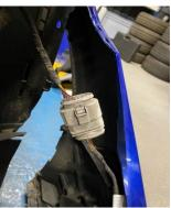
6. You will now need to remove the metal brace on top of the headlights going from the radiator pack to the wing by removing the five T25 bolts securing it in place. You will need to do this on both sides, so make sure to have something in place to support the bonnet and be aware that the headlights will now be loose. Also remove the T25 bolt from the top of the headlight bracket and then unplug the wiring going to the bonnet latches.
