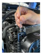
14. Refit the plastic tabs onto the new intercooler and reinstall the radiator cradle in reverse to Step 11. Then push the tabs back through the cradle and use the supplied self-tapper screws with washers to fully secure the intercooler in place, as shown.
