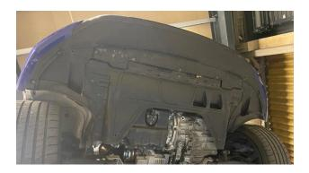
5. The final fixing points for the front bumper are the six T20 bolts on top of the where the grille was located. You can now remove the front bumper and whilst doing so, unplug the wiring harness on the right-hand side of the bumper.
