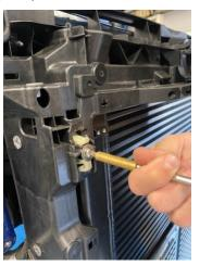
15. Install the supplied aluminium hose joiner into the short silicone pipe and then fit into the longer leg of the supplied 90-degree hose, as shown, and tighten the supplied jubilee clips.
