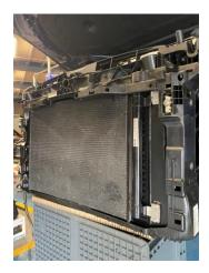
18. Finally, refit the crash bar, headlights, front bumper, arch liners and grille in reverse of Steps 1 to 10 and check everything is tight.
