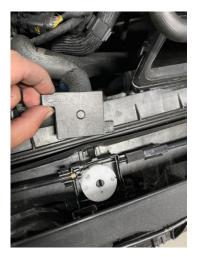
9. Remove the crash bar by unplugging the temperature sensor and horn. Then remove the eight 15mm bolts and four T25 bolts.
