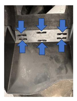
8. Install your new AIRTEC Motorsport air guide by using one of the supplied M6x16 bolts with a Nyloc nut and washers through the slot in the undertray and tighten. On the other side, mark where the slot on the bracket is on the undertray (highlighted with blue arrow) and then make a hole using a 6mm drill bit. You can then install the last bolt and tighten before reinstalling the undertray onto the car.
