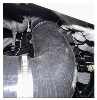
4. Fit the intercooler in place by locating the supplied M12x25mm bolt through the unused tab in the gearbox, as shown, and tighten. Then you can attach the 90-degree hose and once happy with the fitment, tighten the jubilee clips.
