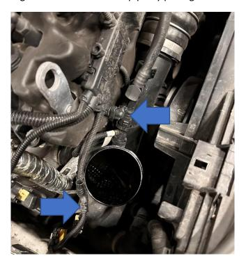
5. You will need to remove the spring clip highlighted. Use a flat-bladed screwdriver or similar to lift up the centre of the clip and then pull it upwards to release it. Once it is removed you can then pull the turbo elbow off.
