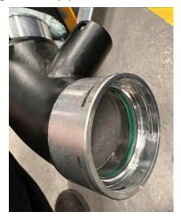
7. Finally, reinstall the new inlet onto the car reusing the spring clip and making sure it is fully seated in the groove. Once happy with the fitment you can reinstall the components removed in Steps 1 to 4 in reverse of removal.
