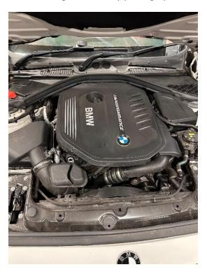
2. Unplug the MAF sensor and undo the jubilee clip. The air box can then be removed by firmly but carefully pulling it up at the corners to release it from its rubber mounts.
