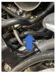
18. Now install the longer silicone hose onto the bottom of the new radiator using the supplied jubilee clip. The 90-degree bend fits nearest to the radiator. Use a P-clip to support it through the bracket, as shown. The hose can then be fed up into the engine bay and then another P-clip will need to be installed onto the existing fuse box stud, as shown.
