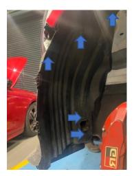
9. With the arch liner removed, you can remove part of the sound deadening as shown.
