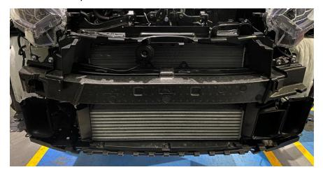
7. You will now need to drain the coolant from the system. To do so, loosen the yellow plug at the bottom of the radiator and allow it to drain. Make sure to have something in place to catch the coolant.
