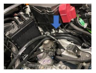
19. Install a hose joiner onto the connection at the back of the engine left from removing the hose in step 17. Use the original clip to secure the connector and then use the supplied jubilee clip to secure to the new silicone hose.
