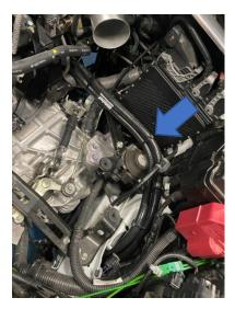
21. Finally, check that everything has been tightened and secured correctly. You can now also add the coolant back and bleed the system. Make sure to check the coolant level to add any additional coolant if necessary. Then refit the air box/intake, arch liners, front bumper and undertray in reverse of removal.
