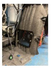
12. Remove the fog light from the side that will have the radiator in place by undoing the three screws on the rear of the light as well as the two screws above the light which hold the surround in place. Once removed, you can apply pressure to the black clips and pull the surround out. Then install the stone guard onto the front using three supplied self-tapping screws. The trim piece can then be refitted in reverse of removal.
