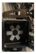
16. Now install the supplied rubber trim around the face of the radiator air guide surround to prevent any rubbing against the bumper.
