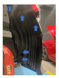
9. With the arch liner removed, you can remove part of the sound deadening as shown.
