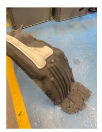
10. You will need to cut the hole for the stone guard. To do so, measure 7cm from the bottom of the arch liner and make a mark for the bottom cut. Then measure 14cm up from that line to find the top mark. You can then measure out a square using four of existing ridges to mark the width, as shown below, and cut out the hole using a sharp knife. Then attach the mounting bracket as shown to ensure fitment.
