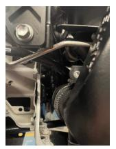
19. The lower hose can now be installed which will pass straight underneath the car and P-clip onto the bottom of the radiator. You can then turn the original hose removed in Step 17 and install the supplied pipe joiner to it and secure using the original clip. Then install the supplied jubilee clip to the silicone hose on the other end.
