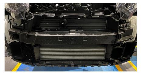
7. You will now need to drain the coolant from the system. To do so, loosen the yellow plug at the bottom of the radiator and allow it to drain. Make sure to have something in place to catch the coolant.
