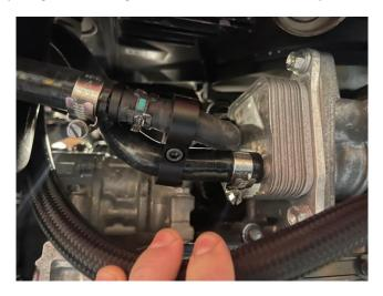
21. Finally, check that everything has been tightened and secured correctly. You can now also add the coolant back and bleed the system. Make sure to check the coolant level to add any additional coolant if necessary. Then refit the air box/intake, arch liners, front bumper and undertray in reverse of removal.
