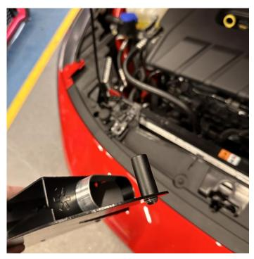
4. On the right-hand side, locate the clip that holds the bonnet release cable and remove it. Then install the air feed in place and lift the cable over the post before refitting the clip. Align both posts with the holes in the car and then install the remaining M6 bolts with washers.
