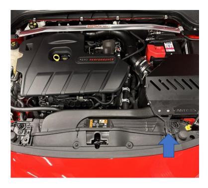
2. Using a trim removal tool, remove the two clips highlighted to allow you to then remove the original air scoop from the car.
