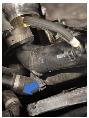
9. You can now remove the spring clip holding the pipe to the turbo. You will need to lift both edges so the clip sits in the groove, as shown. Then lift the centre of the clip to pull it away from the turbo and remove the pipe from the car.
