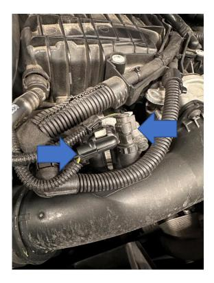
7. Undo the three T27 Torx bolts holding the boost pipe to the throttle body.
