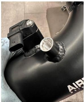
11. Remove the O-ring and clip from inside the original pipe and install onto your new pipe. You will need a flat-bladed screw driver to lift the black plastic part of the clip away from the original pipe but this part is not used on the new one.
