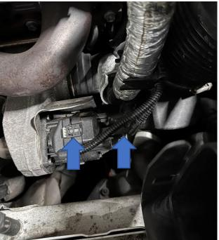
3. Undo the jubilee clip holding the intake hose onto the original turbo inlet and remove the pipe from the car.
