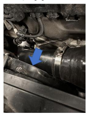
13. Place the second supplied jubilee clip onto the silicone hose and then install the upper part of the boost pipe and using the supplied M6 bolts and washers, tighten onto the throttle body. The weld around the flange can mean that the washer will start to deform as you tighten the top left bolt however this is perfectly fine.
