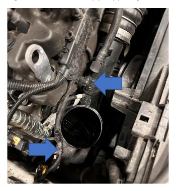
5. You will need to remove the spring clip highlighted. Use a flat-bladed screwdriver or similar to lift up the centre of the clip and then pull it upwards to release it. Once it is removed you can then pull the turbo elbow off.
