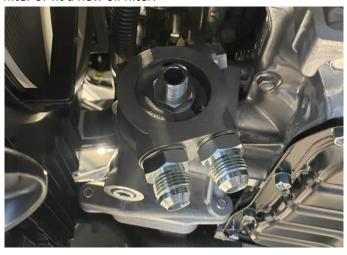
16. Now install the oil lines. The shorter line goes to the left-hand side of the cooler and feeds through underneath the headlight to the sandwich plate fitting nearest the front of the car, as pictured. The longer one goes from the right-hand side to the rear sandwich plate fitting.
