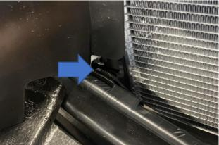
9. Remove the original plastic air guide from above the crash bar by releasing the plastic clips.
