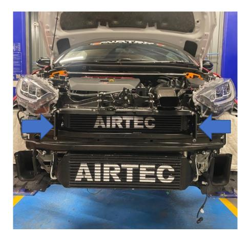
18. **IMPORTANT**: Finally, top up the oil (approx. 500ml) and start the car. Look immediately for leaks from any of the four connections and the oil filter. If so, turn the engine off and retighten the fittings if needed. Then let the car get to full operating temperature, recheck the oil level and top up if required.
