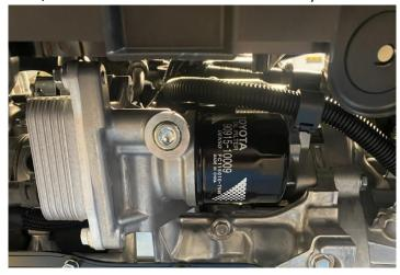
15. Install the sandwich plate using the provided adaptor and fully tighten fittings. Then reinstall the removed oil filter or fit a new oil filter.
