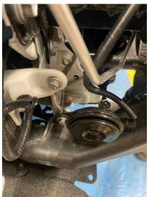
13. Now install the oil cooler by utilising the existing holes either side of the bonnet latch. Secure using the supplied M6x16mm Socket Head bolts with M6 washers and Nyloc nuts.
