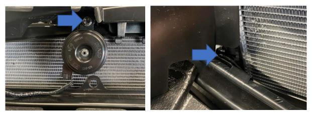
9. Reinstall the horn in the position shown below using the M6 Hex Head bolt and Nyloc nut with washers.
