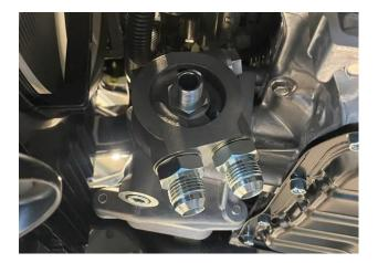
15. Install the oil lines following the route as shown. Then install the oil line separators in the approximate places shown to help keep the lines together (you can twist or move these if needed to help with fitment). Then tighten the fittings onto the oil cooler and onto the sandwich plate. Use either a specific aluminium spanner for AN10 fittings or we would recommend covering an adjustable spanner with masking tape to avoid marking the fitting.
