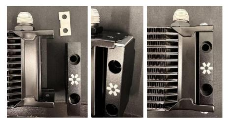
12. Mount the oil cooler to the car using the supplied M8 bolts to go through the mounting blocks to the brackets installed earlier. Once happy with the positioning ensure all the oil cooler bolts are tight.
