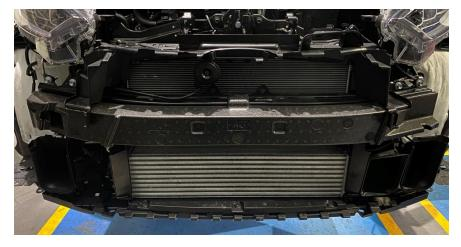
7. Remove the lower plastic trim by removing the three plastic clips using a trim removal tool.
