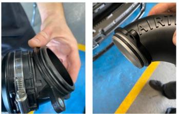
4. Finally, you can now install the AIRTEC Motorsport turbo elbow in place by reusing the two T25 bolts then reinstall the induction hose in reverse of Step 1.
