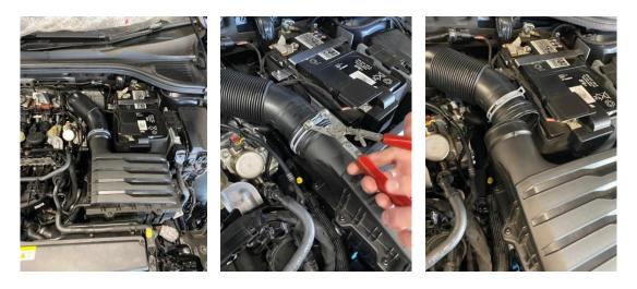
2. At the rear, locate and remove the two T25 Torx bolts securing the original elbow and then remove it together with the induction hose from the engine bay.
