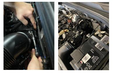
3. Remove the O-ring from the original elbow and transfer it over to the AIRTEC Motorsport item. Then loosen the jubilee clip from the induction hose and remove the elbow.
